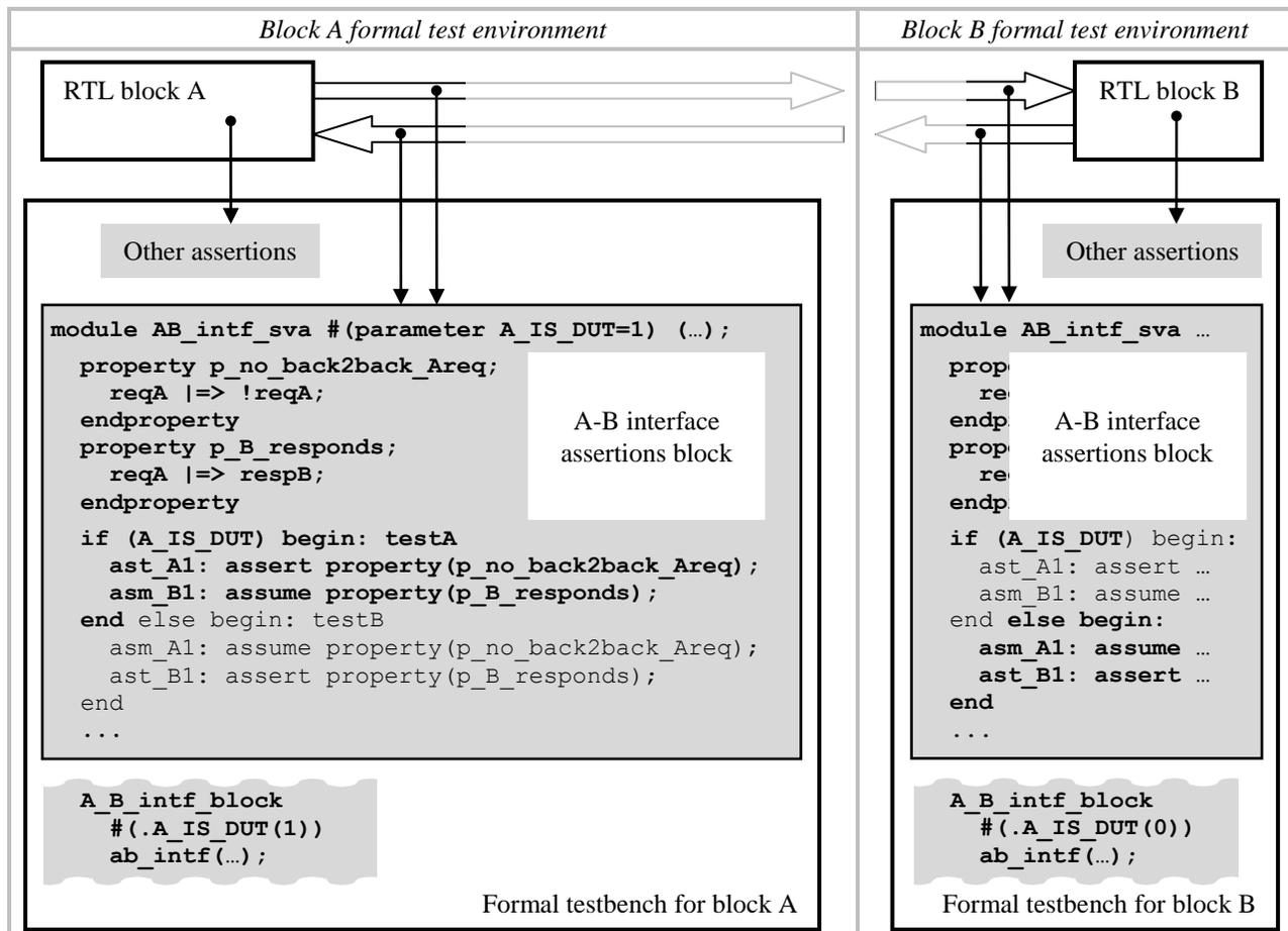
Figure 1: Reversible interface block implements assume-guarantee on a block-to-block interface
